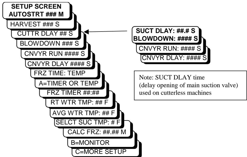
To change the value of a variable, scroll to that line, press the “SET” button on the interface, enter the new value using the numeric key pad and press “ENTER” to accept the new value.
