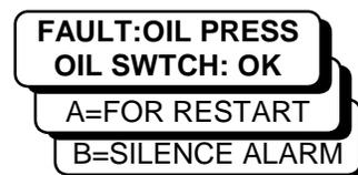
When the oil pressure safety switch has been reset the interface will display "OIL SWITCH: OK". It will be necessary to press "A" on the operator interface to restart the machine.
