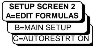
Press “A” to proceed to the Freeze time formula page, SETUP SCREEN 3. Here you will enter the constants for T1; freeze times base on the suction temp, T1.
