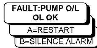
When the overload has been reset the interface will display "OL OK". It will be necessary to press "A" on the operator interface to restart the machine. The cutter overload fault display operates identically to the pump overload displays.
