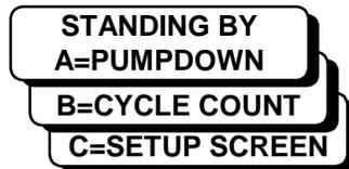
Pressing “A” on the operator interface at this point will cause the machine to begin a pumpdown sequence.
