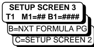
This screen is were the constants, m1 & b1 are entered for a given suction temp, T1. Freeze cycle time will be determined using the linear equation  $y=mx+b$ .
