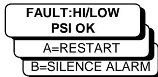
After the safety switch is reset it will be necessary to press the "A" button on the operator interface to return to the start up screen. Pressing "B" on the operator interface at this time will open the alarm contacts.
