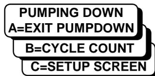
Press the “A” button on the interface to exit the pumpdown mode.
