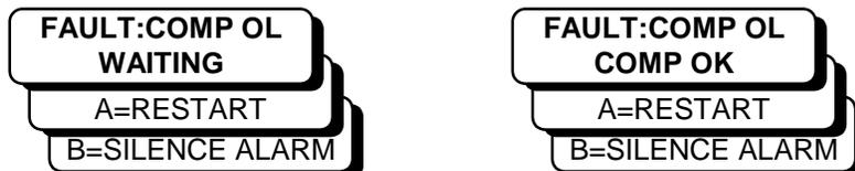
When the compressor overload resets the interface will display “COMP OK”. It will be necessary to press “A” on the operator interface to restart the machine.
