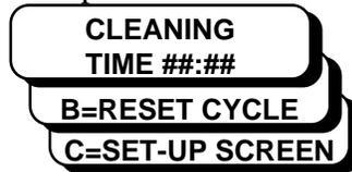
The machine will automatically exit the clean cycle after a 2 hour period. At the completion of the clean cycle the interface will always return to the start up display, requiring that the start button be depressed
