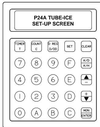
**Figure 10-2, Operator Interface
