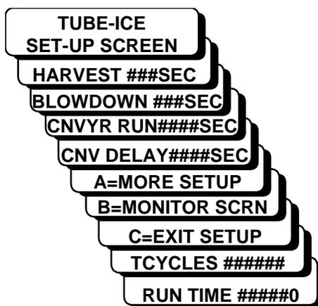
To change the value of a variable, scroll to that variable on the screen, press the “SET” button on the interface, enter the new value using the numeric key pad and press “ENTER”. The only variables that can be changed from this screen are the harvest time, blowdown time, conveyor run time, and conveyor delay time. The last two lines of the display report total cycles and run time of the machine.
