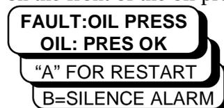
When the oil pressure safety switch has been reset the interface will display "OIL: PRES OK". It will be necessary to press "A" on the operator interface to restart the machine.
