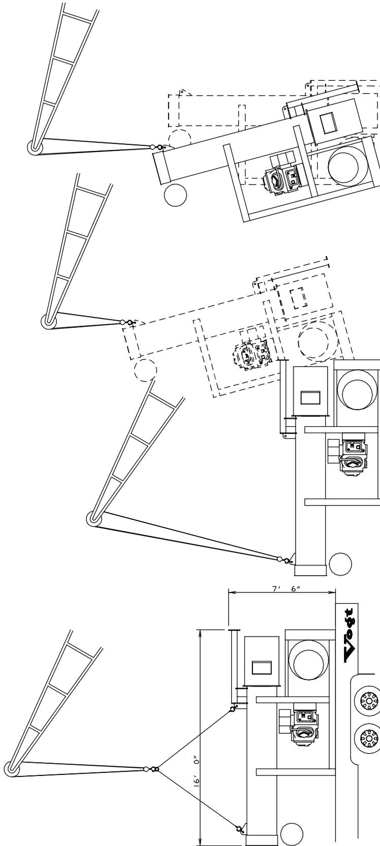
LIFTING MACHINE FROM TRUCK
