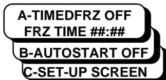
Pressing “A” from this screen will toggle the timed freeze feature from off to on. If the display reads “A-TIMEDFRZ ON” the timed freeze feature is active.
