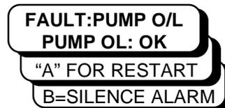
When the overload has been reset the interface will display "PUMP OL: OK". It will be necessary to press "A" on the operator interface to restart the machine. The cutter overload fault display operates identically to the pump overload displays.
