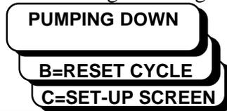
Upon completion of the pumpdown sequence the interface will display the message shown below. It will be necessary to press the start button to resume operation. This screen will also appear upon completion of a clean cycle or after a fault has been detected and reset. The words “PUMPED DOWN?YES” will appear if the machine is pumped down.
