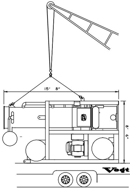
LIFTING MACHINE FROM TRUCK
