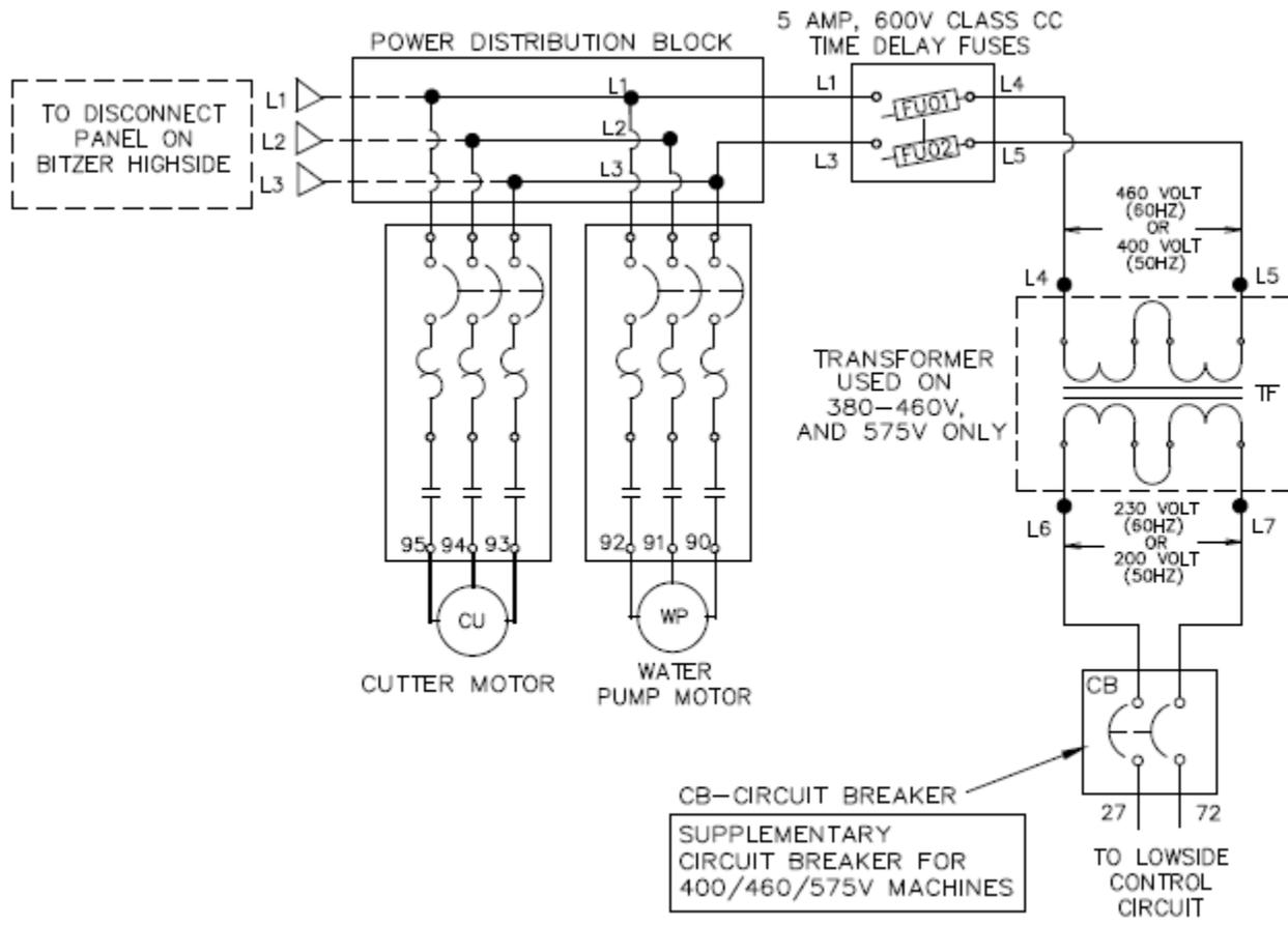
Figure 18: Electrical Schematic, 3-Phase Power, All Voltages 60 Hz
