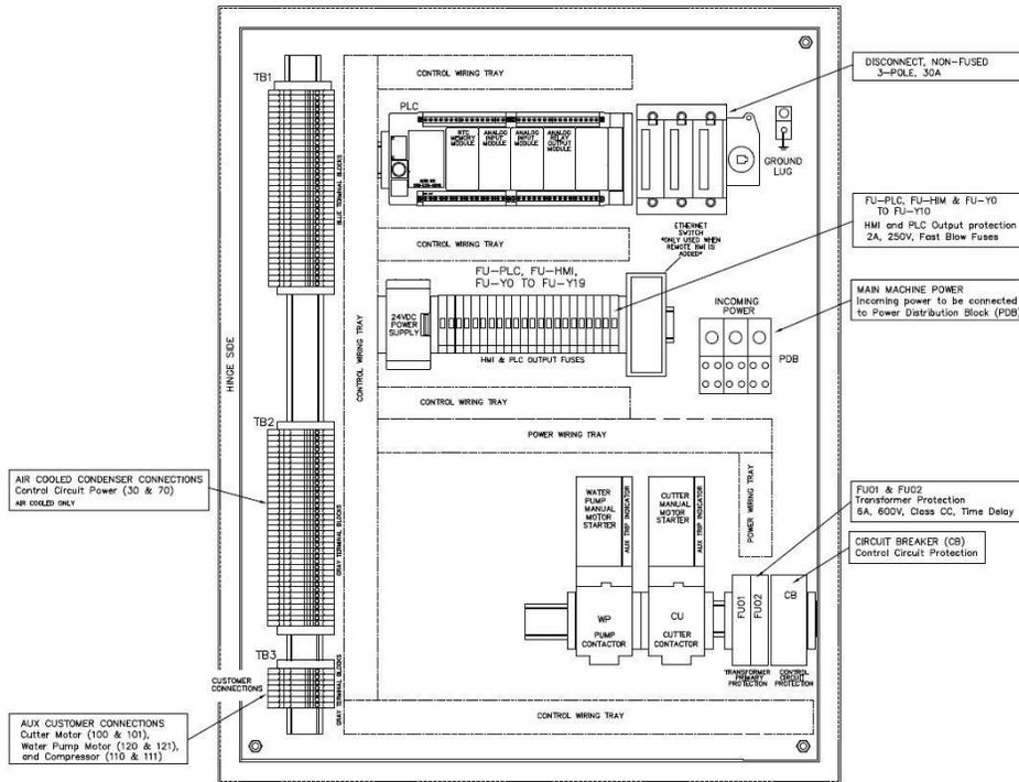
**Figure 13: Control Panel Power Connections (60 Hz)**
