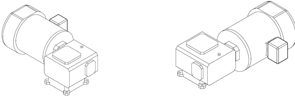
**Figure 74: Cutter Motor and Gear Reducer**
