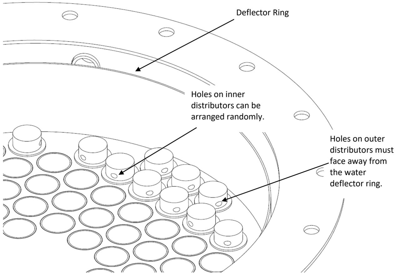
**Figure 66: Water Distributor Detail (Vent Tubes not Shown)**
