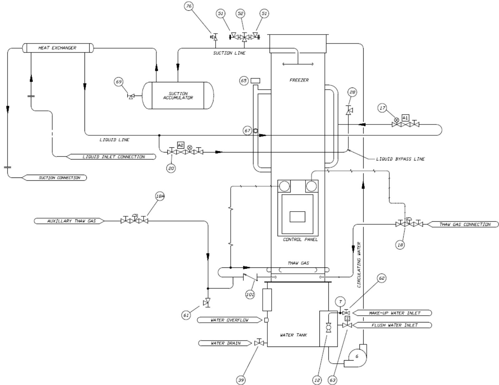
Figure 3: P34HL Low Side Only Piping Schematic
