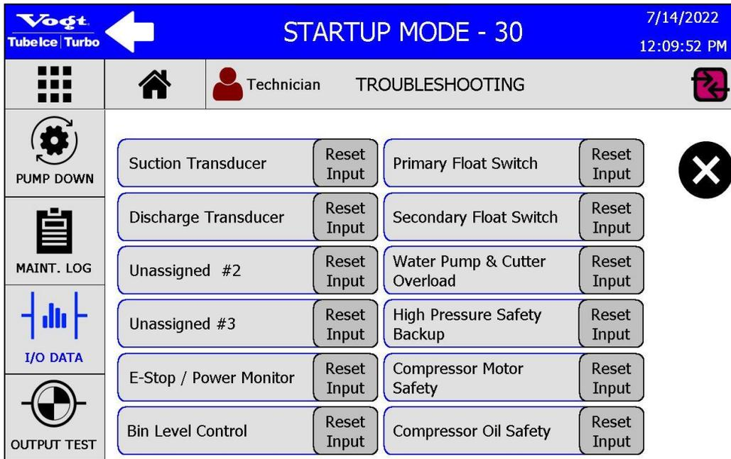
Figure 52: I/O DATA Screen – Input Reset
