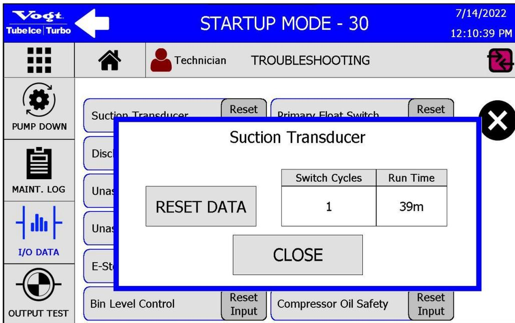
Figure 53: I/O DATA Screen – Input Reset
