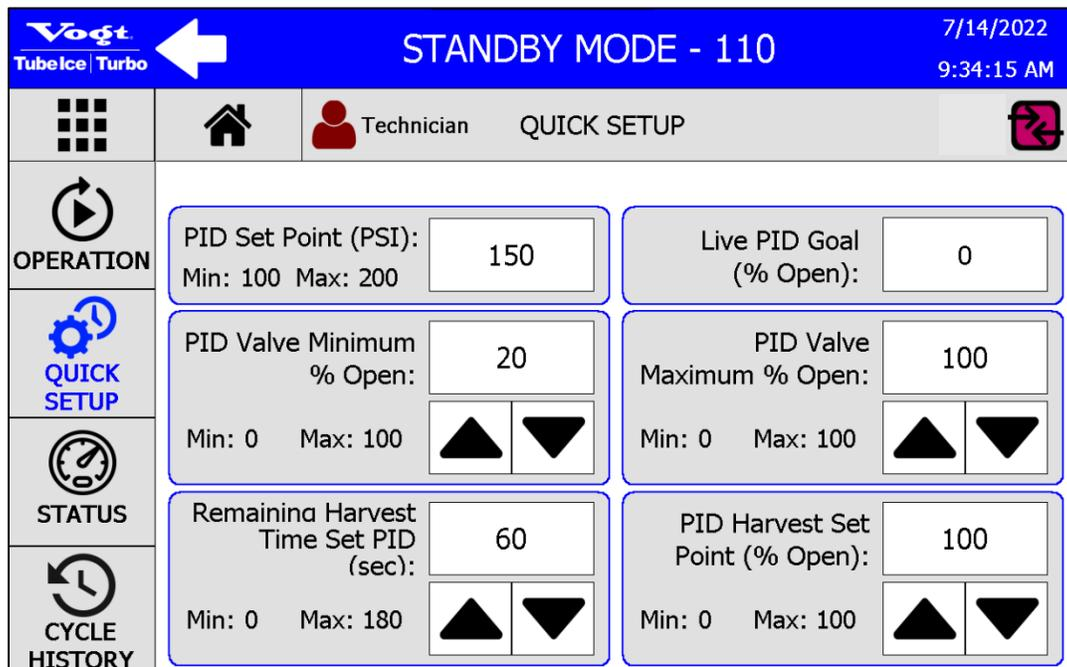
Figure 35: QUICK SETUP – Condenser Water Regulator PID
