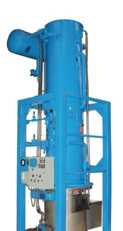
The P34AL Series with a capacity of 50 tons of ice per day is an ammonia low-side Tube-Ice machine designed to operate with a dedicated ammonia high-side or on a central refrigeration system. The P34AL will provide you with many years of dependable service.
