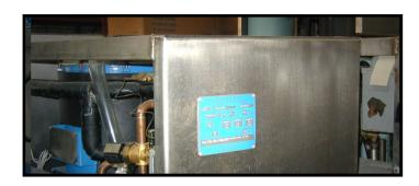
Serial Number Data Code: In 1989, Vogt began adding a date code to the serial number of the ice machine. The code consists of three characters at the beginning of the serial number, two numbers and one letter. These digits depict the year and month of manufacture (89A = January 1989)
