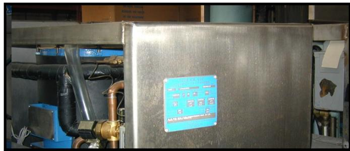
**Serial Number Data Code:** In 1989, Vogt began adding a date code to the serial number of the ice machine. The code consists of three characters at the beginning of the serial number, two numbers and one letter. These digits depict the year and month of manufacture (89A = January 1989)
