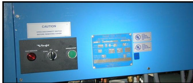
The HES Series control panel was upgraded to a Hoffman enclosure in 2010. The serial number nameplate is located on the upper right corner of the control panel door as shown below.
